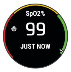
**NOTE:** If you are too active for the watch to determine your oxygen saturation, dashes appear instead of a percentage. You should remain stationary for up to 30 seconds while the watch reads your blood oxygen saturation.
